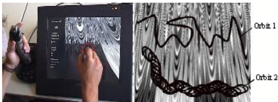
Fig. 1. Left: the scratched gestural control using a tablet and a joystick. Right, two orbits created by direct control (orbit 1) and by parametric control (orbit 2).
